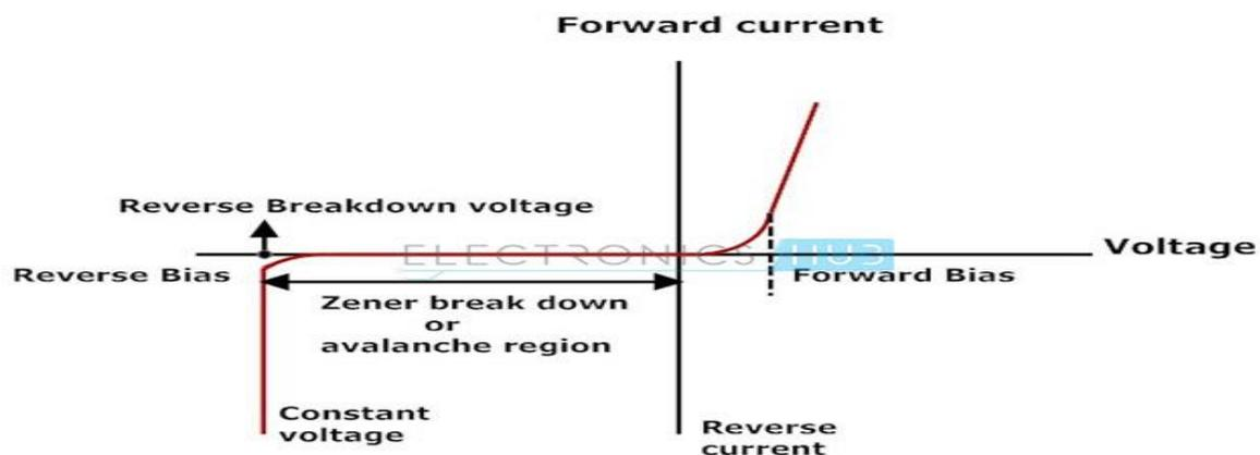
Generally these zener diodes are used to regulate the voltage. In reverse bias condition after the break down zener diode provides a constant output voltage even if we increase the input voltage. There are specifically two separate mechanisms that might cause a breakdown in a zener diode:
