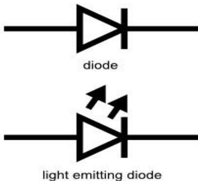
In forward biased, energy is released in the form of light when free electrons in conduction band recombines with holes in the valence band. This process is called electroluminescence. Like a normal p-n junction diode allows electric current only in direction, LEDs also operates only in forward bias condition. The n-type material should be negatively charged and p-type material should be positively charged to create an LED.
