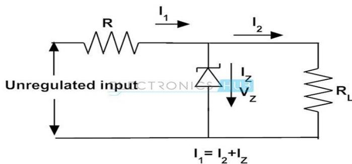
When the load is not connected across the zener diode, no load current will be conducted and all the current due to the circuit will pass through the zener diode dissipating maximum amount of power that causes overheating of the diode and damages permanently.
