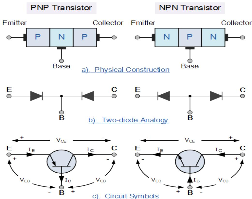
The construction and circuit symbols for both the PNP and NPN bipolar transistor are given above with the arrow in the circuit symbol always showing the direction of “conventional current flow” between the base terminal and its emitter terminal. The direction of the arrow always points from the positive P-
