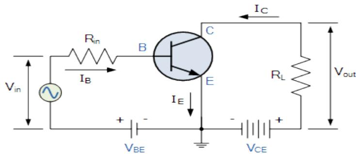
In this type of configuration, the current flowing out of the transistor must be equal to the currents flowing into the transistor as the emitter current is given as  $I_e = I_c + I_b$ .
