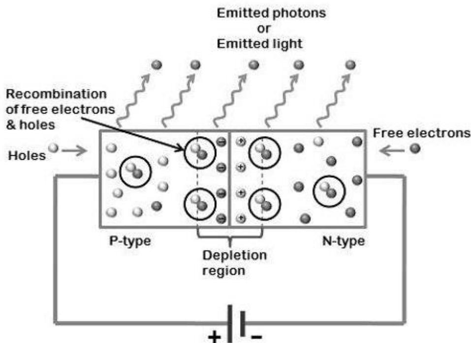
In normal silicon diodes, energy gap between conduction and valence band is less, so low energy photons are released which low frequency and invisible to human eye. Whereas, in LED, energy gap between conduction and valence band is very large so high energy photons released and visible to human eye.
