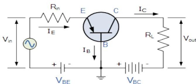
This type of amplifier configuration is a non-inverting voltage amplifier circuit, in that the signal voltages  $V_{in}$  and  $V_{out}$  are “in-phase”. This type of transistor arrangement is not very common due to its unusually high voltage gain characteristics. Its input characteristics represent that of a forward biased diode while the output characteristics represent that of an illuminated photo-diode.
